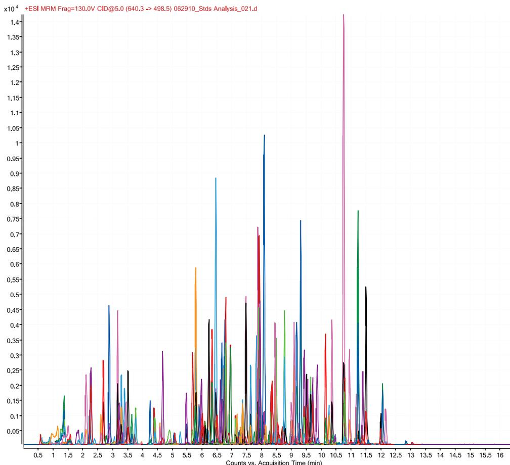
**Figure 7.** Representative overlay mass chromatogram for a 10 ppb ginseng matrix matched standard.
