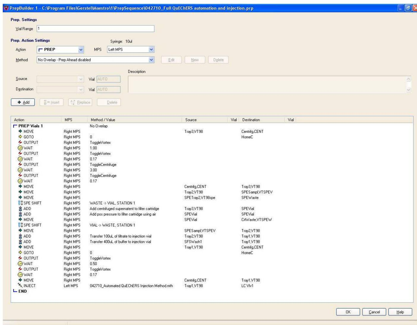
Figure 2. Example Prep Sequence for Automated QuEChERS LCMSMS Analysis.
