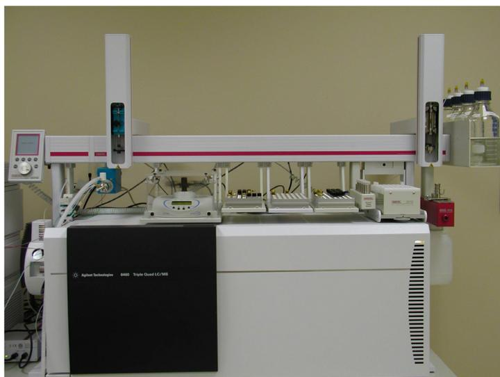
**Figure 1.** MPS 2XL dual head, multi-purpose sampler configured for automated QuEChERS-LC/MS/MS analysis.
