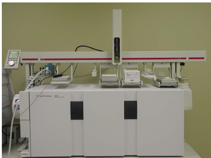
Figure 1. MPS 2XL MultiPurpose Sampler (MPS) with GERSTEL DPX option.
