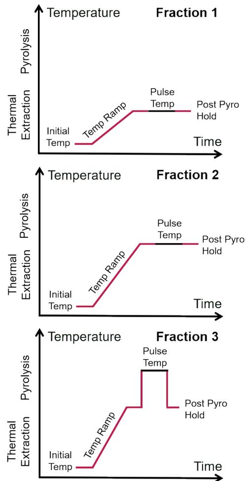
Figure 3: Temperature programs for fractionated pyrolysis (FP) mode
