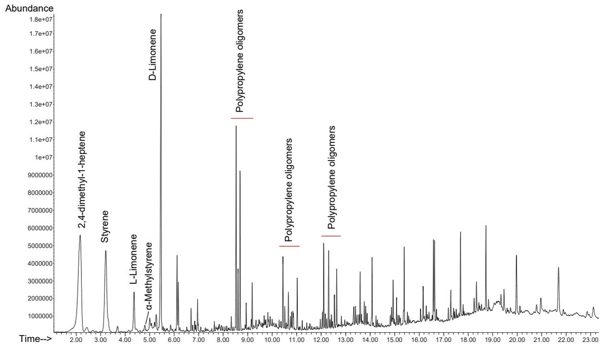
Figure 5: Total Ion Chromatogram resulting from SRP of packaging tape sample
