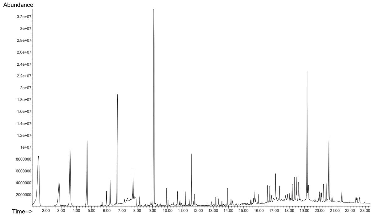
*Figure 6: Total Ion Chromatogram resulting from SRP of mascara sample*
