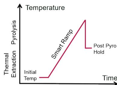
Figure 2: Temperature program for smart-ramped pyrolysis (SRP) mode
