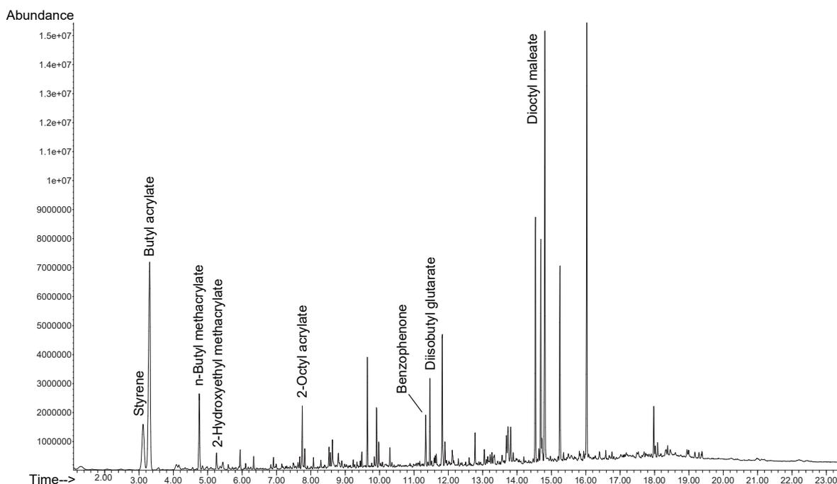
Figure 4: Total Ion Chromatogram resulting from SRP of house paint sample
