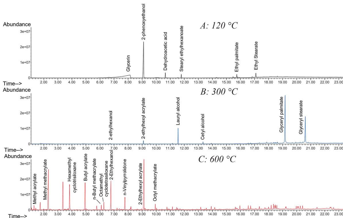
Figure 7: Stacked view for FP of mascara sample at (A) 120 °C, (B) 300 °C and (C) 600 °C.
