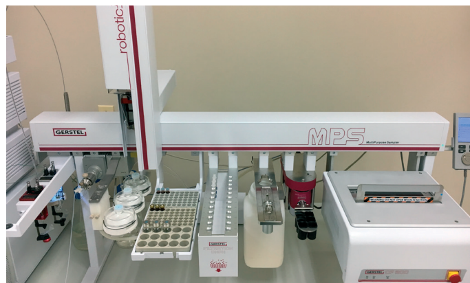
Figure 1: GERSTEL MPS robotic PRO sampler with Agilent LC System. The MPS is configured with Filtration Option, which was not used in this work.
