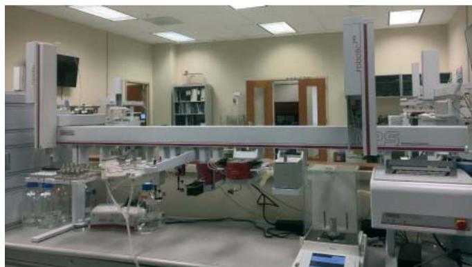
Figure 1. MPS robotic/robotic<sup>PRO</sup> sampler configured with GERSTEL automated sample preparation options.
