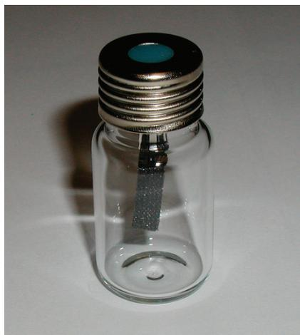
Figure 1. TF-SPME device in 10 mL vial.
