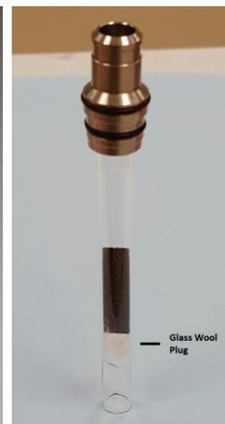
Figure 2. TF-SPME device in TDU tube.
