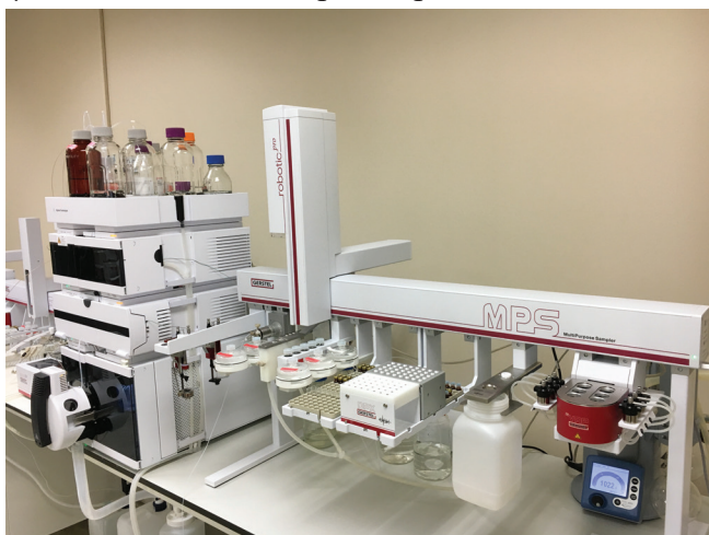
Figure 1. MPS robotic PRO Multi-Purpose sampler with the GERSTEL DPX option.
