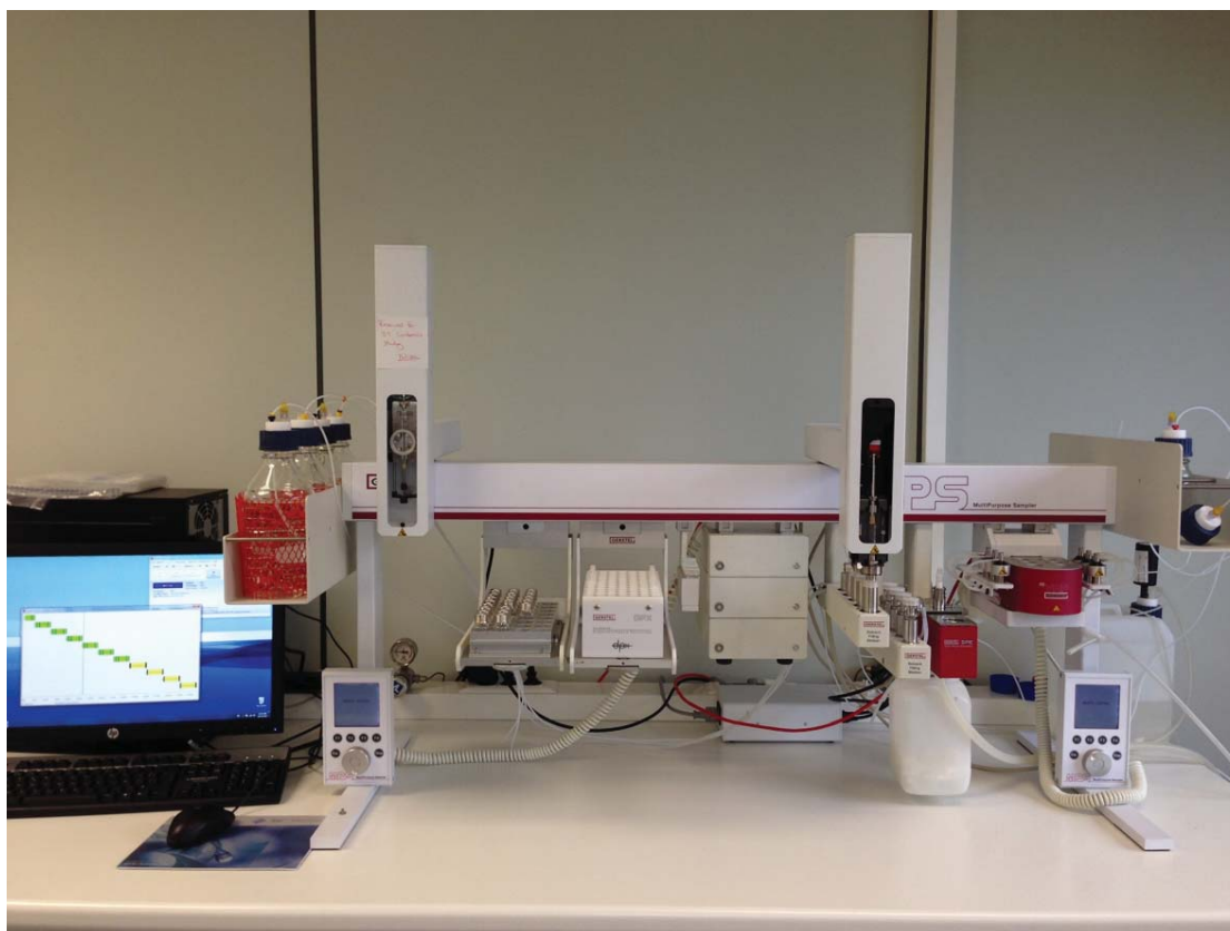
Figure 1. MPS Dual Head WorkStation configured for automated SPE and concentration.
