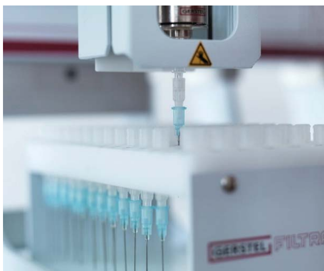
Figure 3. Pictures of the MPS transporting the 0.45 \mu\text{m} filter from the filtration tray (left) to the VT-98 tray with filtration cover (right).
