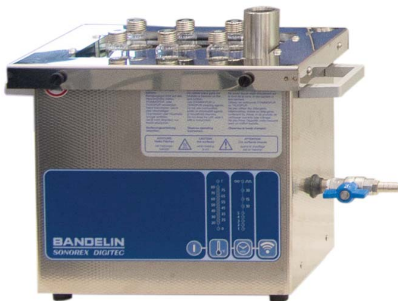
Figure 2. Picture of the ultrasonic bath used for automated ultrasonic extraction of the plant material.
