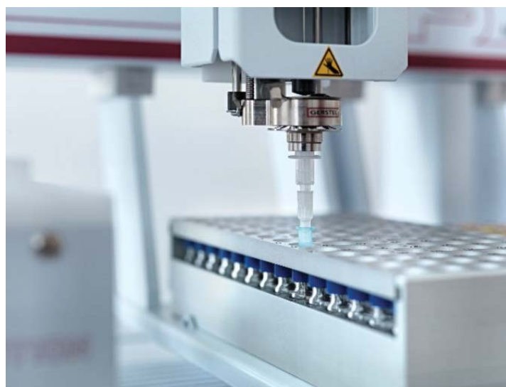
Figure 3. Pictures of the MPS transporting the 0.45 \mu\text{m} filter from the filtration tray (left) to the VT-98 tray with filtration cover (right).
