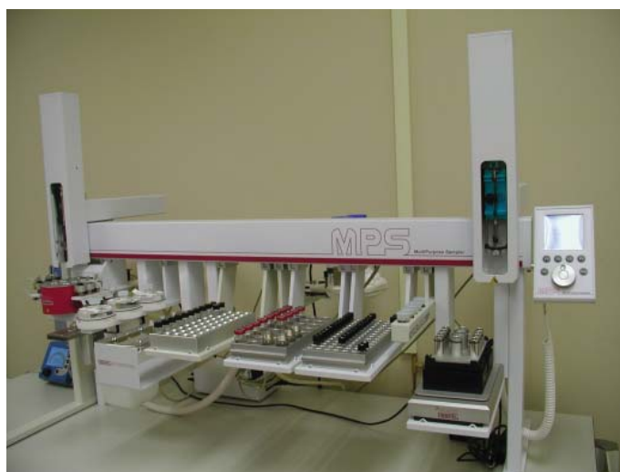
Figure 1. GERSTEL MultiPurpose Sampler (MPS) Dual Head WorkStation configured with mVORX, mVAP, and Universal Filtration Options.
