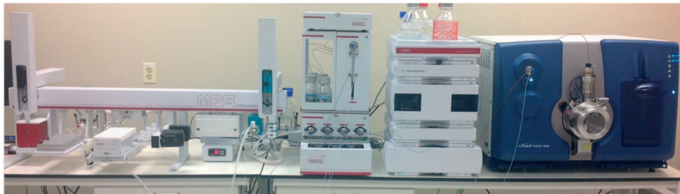
Figure 2. GERSTEL MPS XL with SPE XOS coupled to a QTRAP® 4500 system.
