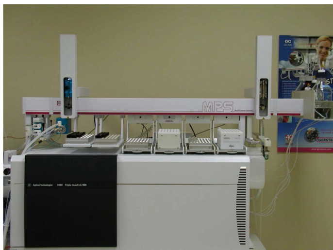
Figure 1. MPS 2XL multi-purpose sampler with the GERSTEL DPX option for high throughput pain management drug screening.
