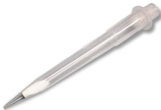
Figure 1. GERSTEL Disposable Pipette Extraction (DPX). Pipette tip with loosely contained sorbent mounted with a transport adapter to facilitate automation.
