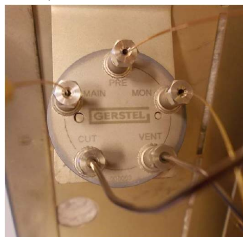
Figure 2. GERSTEL \mu\text{MCS} fraction distribution device.
