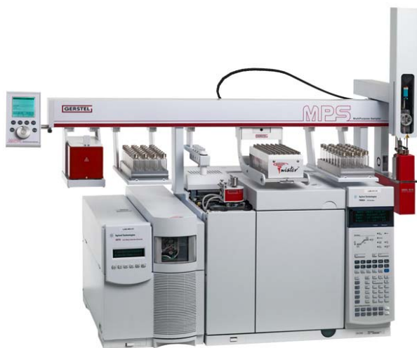
Figure 1. GC/MS system used for automation of all sample introduction techniques.
