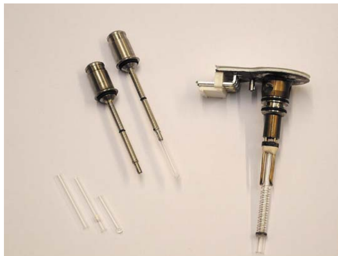
Figure 1b. Pyrolysis Module (PYRO) shown with transport adapters and sample holders.
