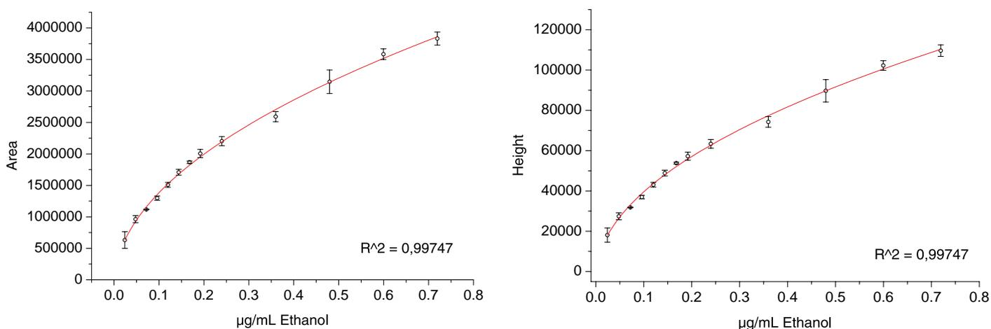
**Figure 8.** Calibration of the Sensor with liquid injection of ethanol in an empty and blank calibration can. Liquid injections varied between 0.01 to 0.3 µL, can volume was 330 mL. The shown error bars result from 3 injections atn each level.
