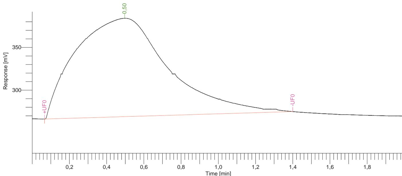
**Figure 7.** Sensor Signal, calibration run with 0.3 µL ethanol added to a 330 mL empty and blank can.
