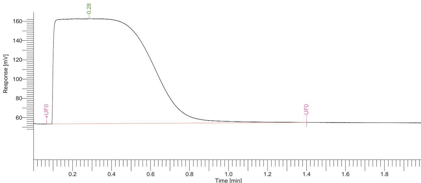
**Figure 5.** FID Signal, calibration run with 0.3 $\mu$ L ethanol added to a 330 mL empty and blank can.
