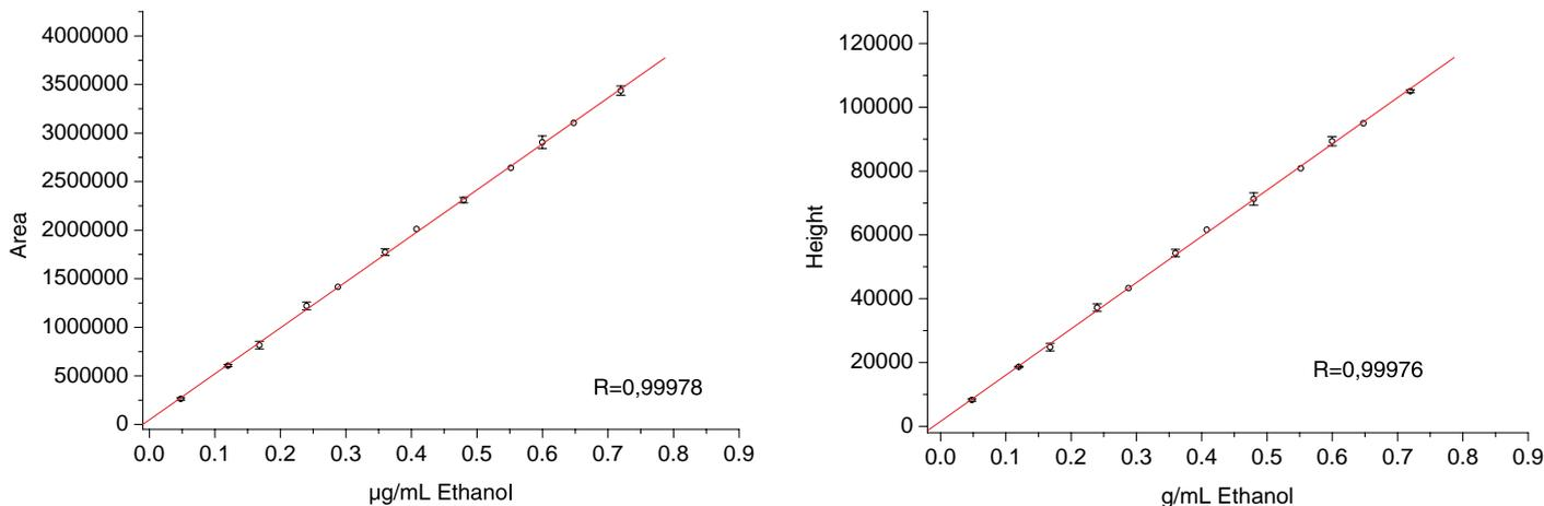
**Figure 6.** Calibration of the FID with liquid injection of ethanol in an empty and blank calibration can. Liquid injections varied between 0.02 to 0.3  $\mu$ L, can volume was 330 mL. The shown error bars result from 2 injections at each level.
