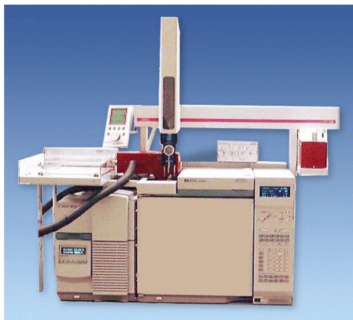
Figure 1. GC/MS system used in the study. SPME autosampler coupled with a septumless head in the front injector and Thermal Desorption Autosampler coupled with a PTV injector in the back injector.
