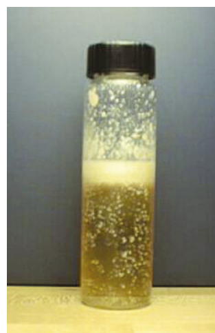
Figure 3. Emulsion formed during solvent extraction of liquid hand soap.
