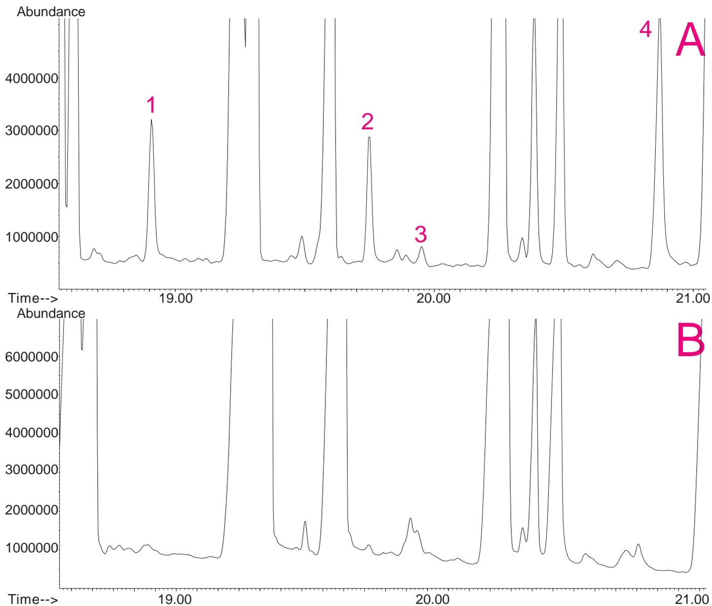
**Figure 2.** Twister extract of water spiked with semi-volatile organic compound (SVOC) mix. (A) acidified (B) non-acidified. Peak identities: 2,3,5,6-tetrachlorophenol (1); 2,4,6-tribromophenol (2); o-(o-bromophenyl)phenol (3); pentachlorophenol (4).
