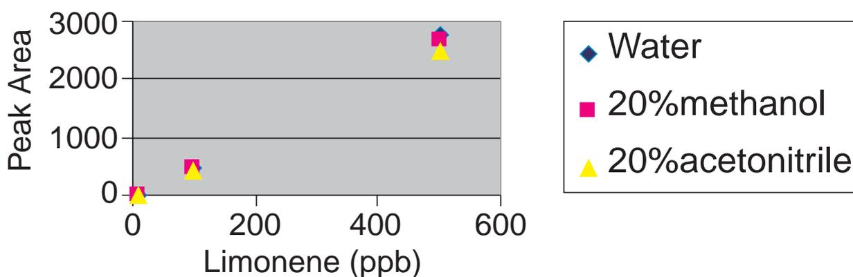
**Figure 4.** Limonene calibration curves. 10mL, Twister extraction, 30:1 split.
