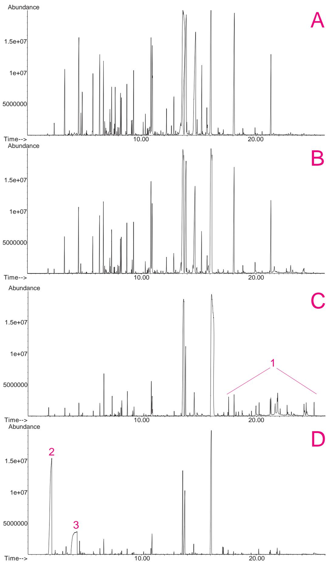
**Figure 7.** Twister extractions of artificial coffee flavor diluted 1:10 with A) water B) 10% acetonitrile C) 30% acetonitrile D) 50% acetonitrile. Peak identities: (1) C16-C18 esters, (2) acetonitrile, (3) propylene glycol.
