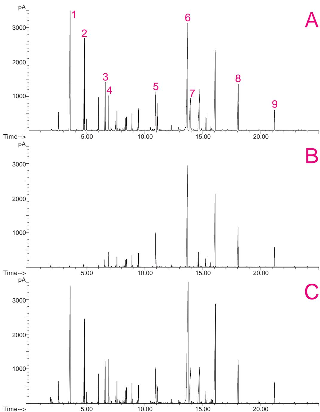
**Figure 5.** Twister extraction of artificial coffee flavor diluted 1:10 in (A) water (C) 10% methanol. (B) Back extraction of Twister with 10% methanol. Peak identities: (1) ethyl propionate, (2) ethyl butyrate, (3) pentyl acetate, (4)  $\alpha$ -pinene, (5) ethyl octanoate, (6) ethyl decanoate, (7) vanillin, (8) benzyl benzoate, (9) benzyl cinnamate.
