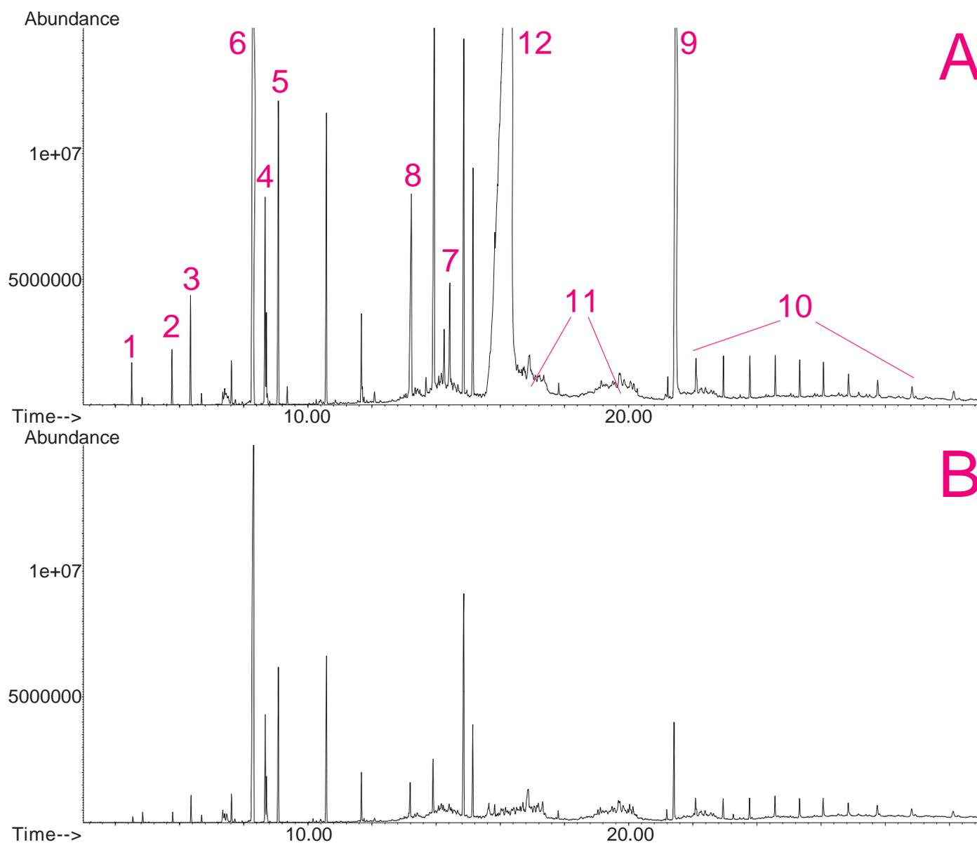
**Figure 3.** Twister extraction of liquid hand soap (A) and after back extraction at pH8 (B). Peak identities: 12) lauric acid, (9) Triclosan, (10) C20-C30 hydrocarbons, (11) polyoxyethylene alcohols or triglycerides, (6) limonene, (7) ethyl vanillin, (1-5) esters and (8) decalactone.
