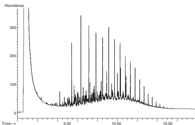
**Figure 2.** Diesel, 1:100 in hexane, without venting.
