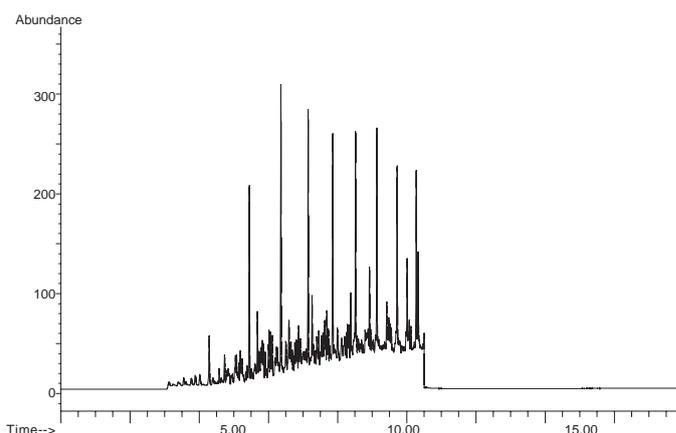
**Figure 3.** Diesel, 1:100 in hexane, venting and back-flush.
