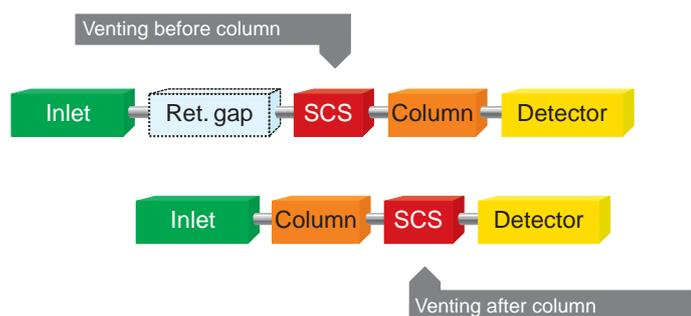
**Figure 1.** Single column switching system SCS.
