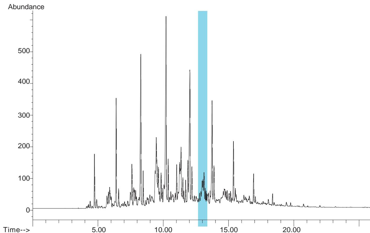
**Figure 12.** Pre-column chromatogram of naphtha, marked compounds transferred.
