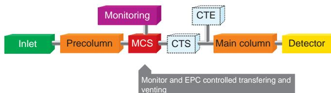
**Figure 9.** Multi column switching system MCS.
