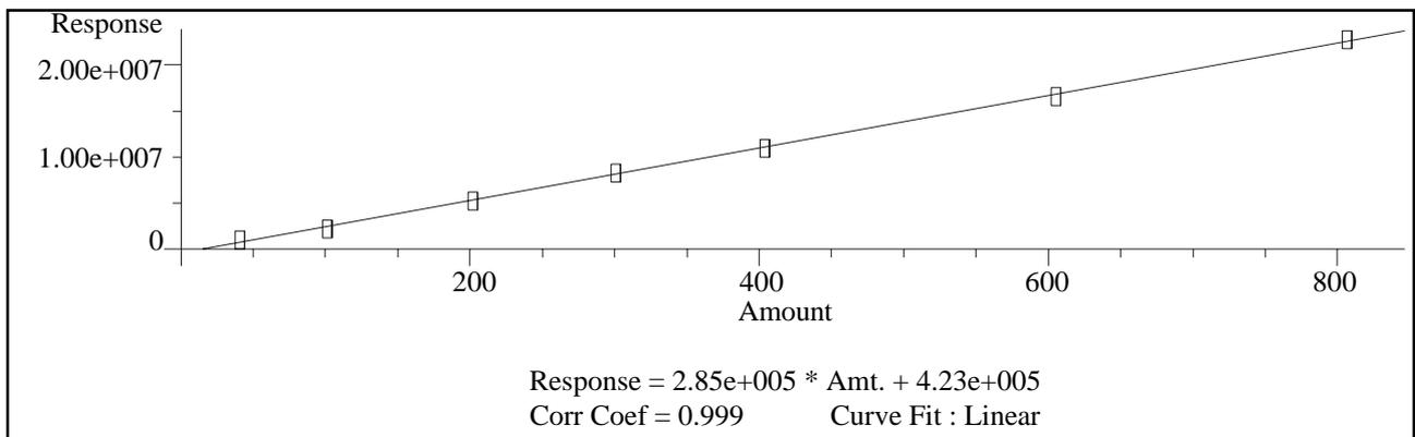
**Figure 5.** *Calibration curve for 4-heptanone in urine.*
