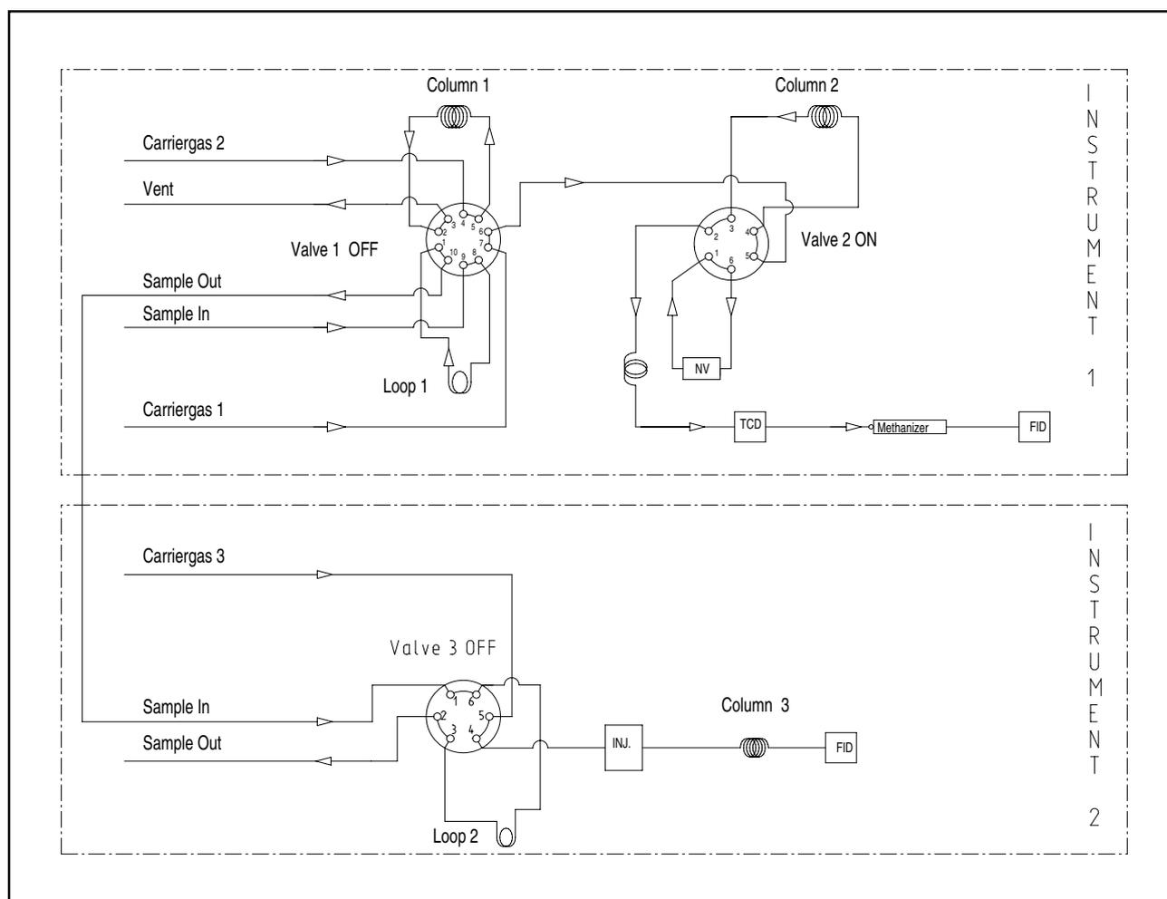
**Figure 1.** Overall schematic design of the heart of the analyzer. Mode: "stand by" or analysis of the components present in column 2 or flushing of the sample loops of both instruments and backflush of column 1.
