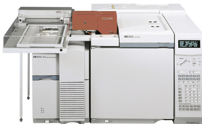
Figure 3. GERSTEL ThermoDesorption ChemSensor System.
