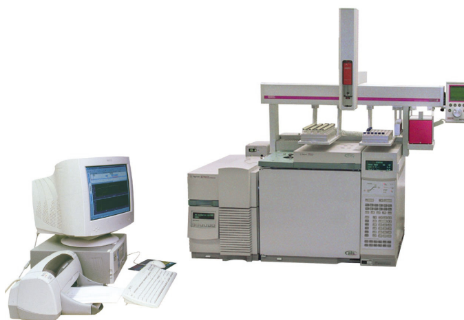
Figure 1. Gerstel Headspace ChemSensor System.
