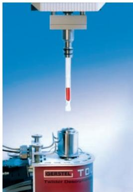
samples can be processed automatically for determination of VOC / SVOC in heavy or involatile matrices. Following the analysis, the sample cup with the remaining high-boiling or solid residue is automatically removed. ATEX helps to ensure maximum uptime and best possible analysis results by keeping involatile or complex matrix material out of the GC/MS system. Standard addition and other
