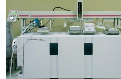
MPS 2XL MultiPurpose Sampler with the GERSTEL DPX Option.
