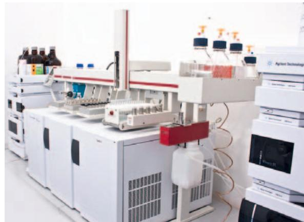
**The SPE LC-MS/MS system used by the TeLA scientists for the pesticide multi-residue method consisting of an Agilent Series LC 1200 and a GERSTEL SPE system mounted over an Agilent 6410 MS/MS Triple Quad.**
