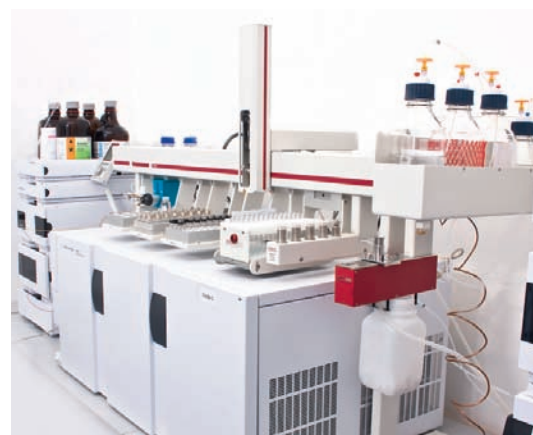
The SPE LC-MS/MS system used by the TeLA scientists for the pesticide multi-residue method consisting of an Agilent Series LC 1200 and a GERSTEL SPE system mounted over an Agilent 6410 MS/MS Triple Quad.
