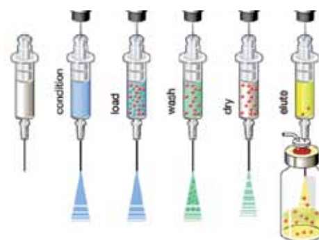
Schematic of GERSTEL automated Solid Phase Extraction (SPE)
