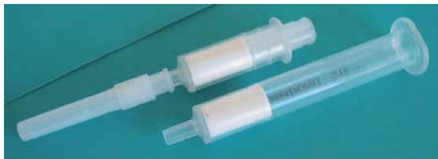
Standard Solid Phase Extraction (SPE) cartridge and same cartridge in GERSTEL format for automation. Cartridges in this format are readily available from several vendors: Agilent, Sigma-Aldrich, Macherey&Nagel and others on request.
