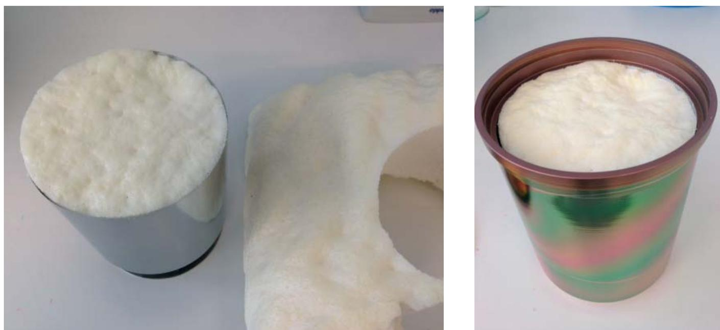
*Figure 3. Custom-made coring tool and sample of the SPF open-cell foam (left) and the coring tool together with the sample, the surface at the top, placed into the one Liter container (right).*
