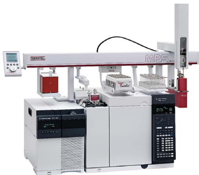
Figure 1. GERSTEL MPS-DHS-TDU Agilent 7890/5977 GC-MSD system.
